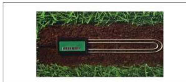
Fig. Soil moisture sensors
